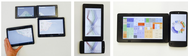
Figure 3. Mock-up of device combinations: simple extension of the graphical context (left, cf. [14]), aligned and extended parallel coordinate plot (center), two different linked visualizations (right).
